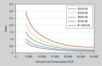
10 MW main engine, 3 x 0.5 MW aux engines. Total investment cost \$3 million.
